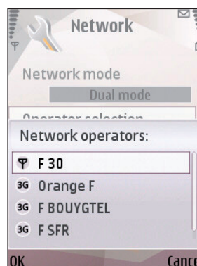
Figure 3: Nokia N95 scanning for local GSM operators. OpenBTS is labelled 'F30'.
