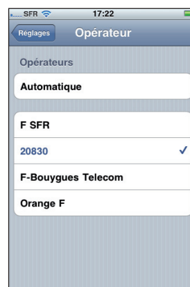
Figure 2: iPhone scanning for local GSM operators. OpenBTS network is labelled '20830'.
